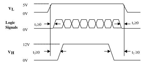
Figure 1. Power Supply and Logic Signal Sequencing
